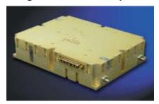
The model SSPA 0.5-2.5-30 is a high power, broadband, gallium nitride (GaN) RF amplifier that operates in a frequency range from 0.5 to 2.5 GHz. This PA is ideal for broadband military platforms as well as commercial applications because it is robust and offers high power over a multi-octave bandwidth. The amplifier operates with a base plate temperature of 85°C
